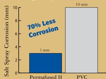
Level of corrosion under color coating after 1,000 hours of exposure to salt spray of scribed sample. Test conducted in compliance with ASTM B 117.
